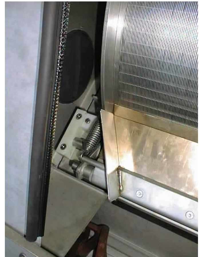
Automatic doctor blade cleaner (double scraper) with tension spring for cleaner blade
